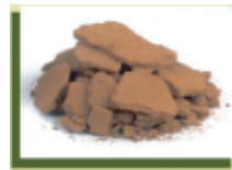
經脱水處理後形成泥餅狀 The sludge cake after dehydrating.
