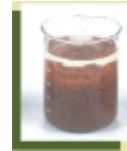
經Polymer加藥調理反應後污泥形成膠羽凝結 Floc coagulation after chemical/polymer conditioning.
