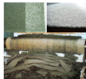
(含油污泥脫水實例) (Example for oil-retaining sludge cake outlet)
